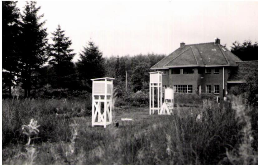
Figure C.1: Thermometer screens at 1.50 m (front) and 2.20 m (back) above ground level at KNMI station Witteveen at 9 September 1958. Photograph taken in west-southwesterly direction
