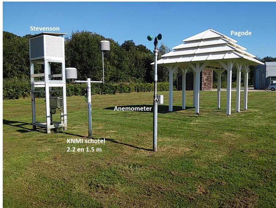
Figure 2.1: Situation of the thermometer screens on the KNMI test field in De Bilt. The KNMI multi-plate screen (KNMI schotel) is double and measures at both 2.20 and 1.50 m above ground level. The measurements of the multi-plated screens are the subject of the present study. The anemometer is at 2.20 m above ground level and is used in the analysis of this report. Photograph is taken in Northerly direction.
