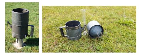
Figure 2.2: Left: KNMI manual rain gauge (collecting surface 200 cm2) consisting of a reservoir (lower part) and a funnel (upper part). Right: Funnel and reservoir taken apart and the measuring cylinder. Before each measurement the funnel is removed from the reservoir and the reservoir is emptied into the measuring cylinder.
