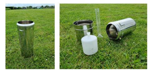
Figure 2.1: Left: Hellmann manual rain gauge (collecting surface 200 cm2) consisting of a reservoir (lower part) and a funnel (upper part). Right: Funnel and reservoir taken apart, the plastic container and the measuring cylinder. For the manual evaluation of the daily precipitation amount, the funnel is removed from the reservoir. Thereafter the container is emptied into the measuring cylinder.
