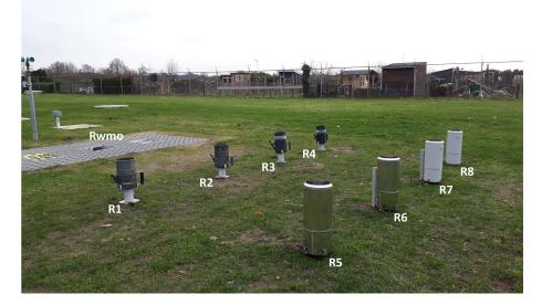
Figure 2.3: Experimental set-up at the KNMI test field in De Bilt. Photograph taken in northeasterly direction. Table 2.1 contains a description of the gauges.
