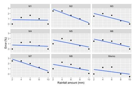
Figure A.1: Error resulting from the measuring cylinders as a function of rainfall amount in the cylinder. M1 corresponds the the measuring cylinder of R1, M2 of R2, etc. The straight line represents a linear regression fit.
