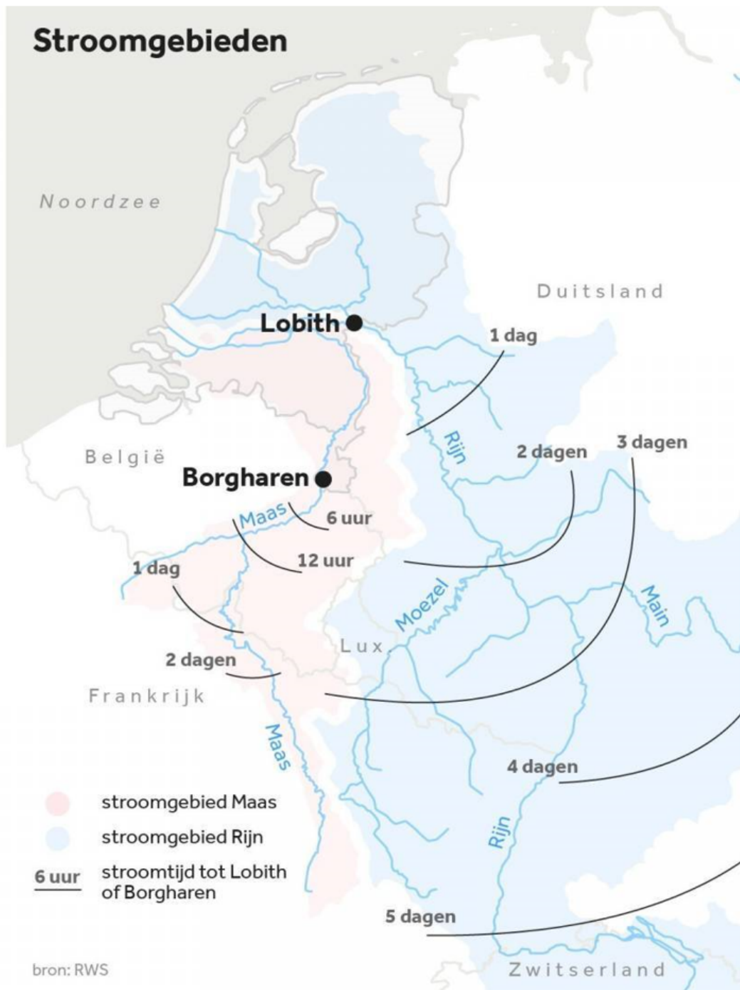
Figure 1.4: Indication of the runtimes of the Meuse and the Rhine at the Dutch border to upstream rainfall events. The response times will be larger than the runtimes.
