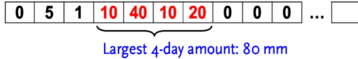
Figure 1.2: Explanation of the resampling methodology in the weather generator (Hegnauer et al., 2014)
