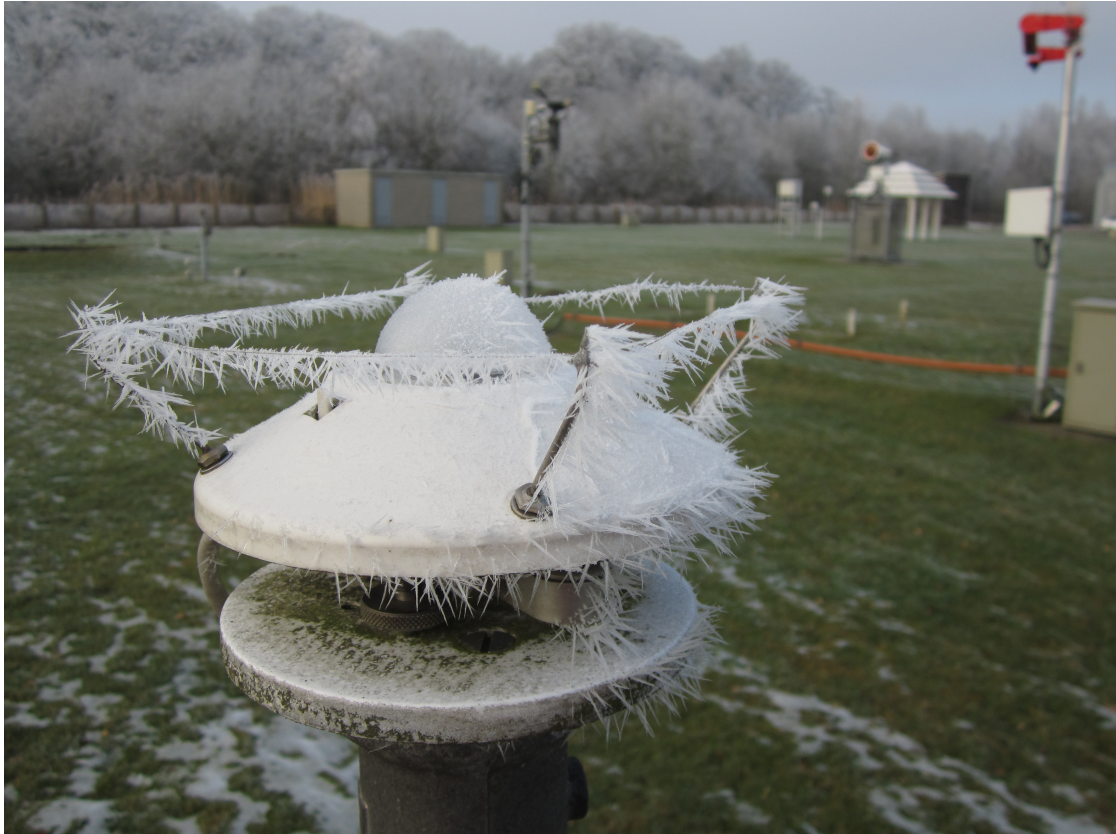
Figure 4.14: Heavy rime on a Kipp & Zonen CM-11. The photo was not taken during the intercomparison.
