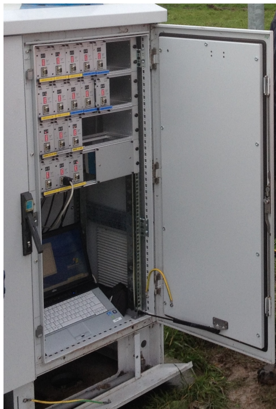
Figure 2.5: Cabinet with electronics. Inside the cabinet, four racks with SIAMs are visible, that provide the data acquisition for the entire BSRN site.
