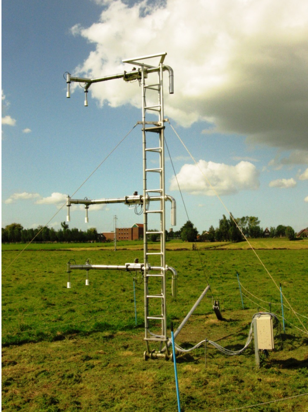
Figure 7 Bowen ratio system at Energy Balance terrain with psychrometers at 1, 2 and 4 m above the surface.
