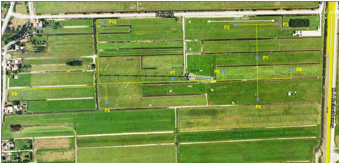
Figure 9 The position of the micro-barameters. To the right is the basic pentagon (P2-P6, with 1 in the center), to the left are additional sensors (P7-P10) to extend the baseline length. The coordinates are given here (pdf) . For the Five other micro barographs (P11-P15) are positioned in the 200-m tower at 60, 100, 140, 180 and 200m respectively. For the layout see here (pdf) .
