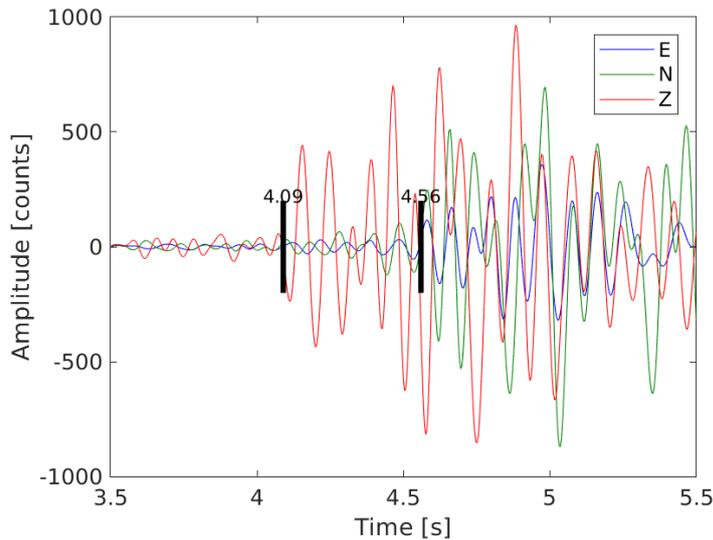
Figure 11: 3-component response at accelerometer RBF, at a time window around the first P- and S-wave. The black bars denote the picked onset times of the first P- and S-wave, at 4.09 and 4.56 s, respectively.
