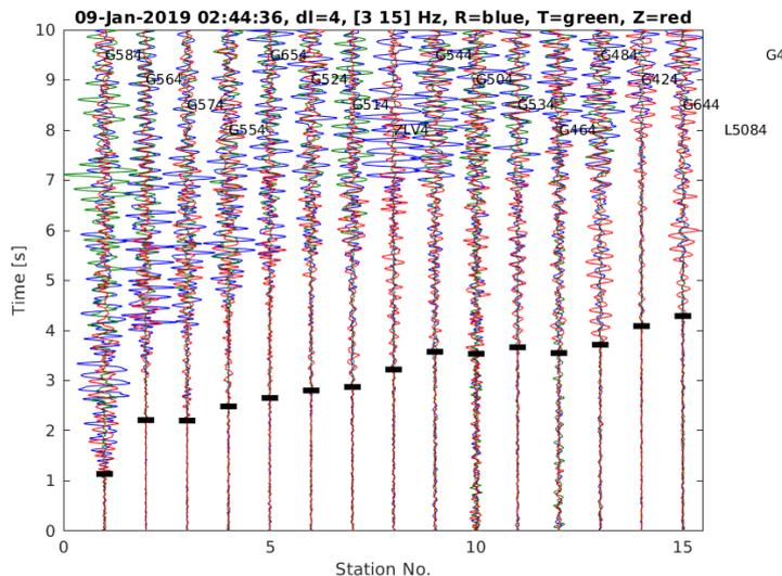
Figure 5: Event gather for Veendam event for the 13 nearest 200-m depth stations from the KNMI network. The 3 colours show recordings over 3 orthogonal components: radial (blue), transverse (green) and vertical (red). P-wave onset picks are indicated with black bars. The underlying waveform data is publicly available and can be obtained through <http://rdsa.knmi.nl/dataportal/> or <http://rdsa.knmi.nl/fdsnws/dataselect/1/>.
