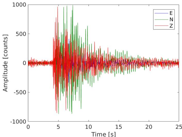
Figure 9: 3-component response at accelerometer RBF, which is located at [lat, lon]=[53.08274 6.9337]. The 3 colours show recordings over 3 orthogonal components: east (blue), north (green) and vertical (red).
