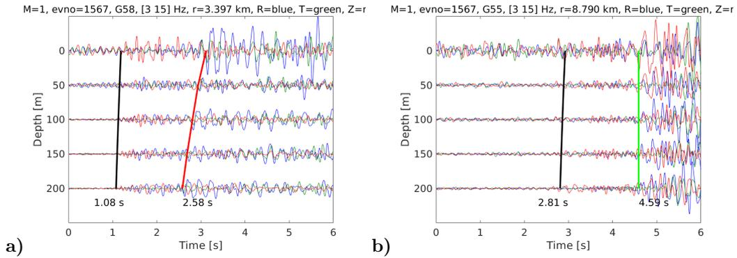
Figure 10: 3-component response at 5 depth levels in boreholes (a) G58 and (b) G55. The red, blue and green seismograms denote the vertical, radial and transverse particle velocity recordings. Thick black and red lines denote depth-consistent picks of the first P- and S-wave onset, respectively. The green line shows the simultaneous arrival time of the guided wave at the different sensor levels.
