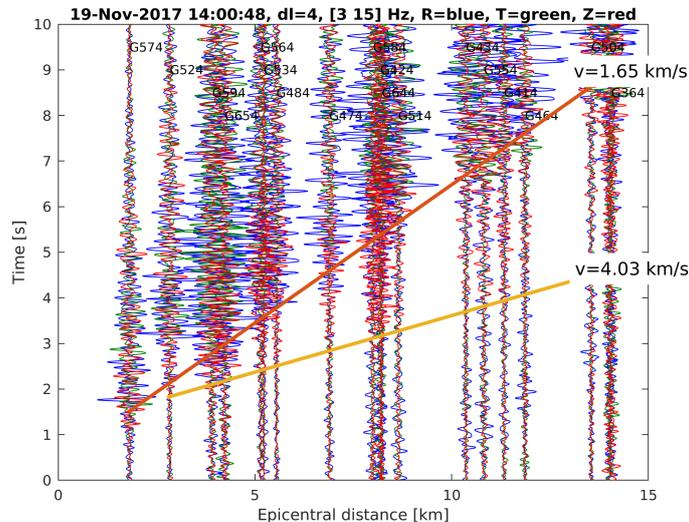
Figure 4: Event gather of Winschoten 19-11-2017 event. The 3 colours show recordings over 3 orthogonal components: radial (blue), transverse (green) and vertical (red). The two straight lines depict fits of the two most prominent arrivals. The slope of the lines correspond to the indicated velocities.
