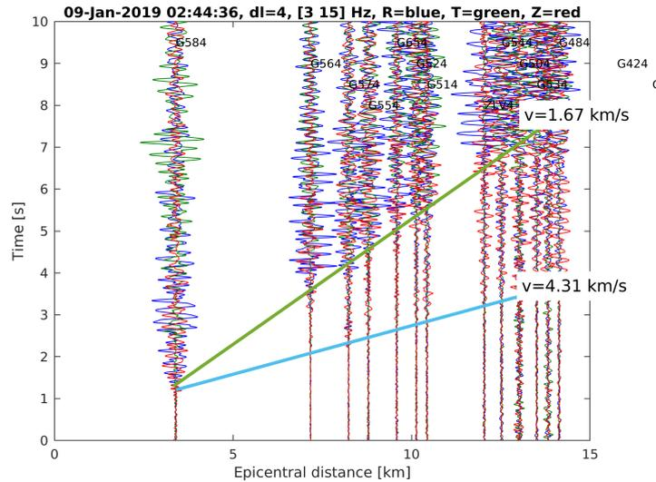
Figure 1: Event gather of Veendam 09-01-2019 event. The 3 colours show recordings over 3 orthogonal components: radial (blue), transverse (green) and vertical (red). The two straight lines depict fits of the two most prominent arrivals. The slope of the lines correspond to the indicated velocities.
