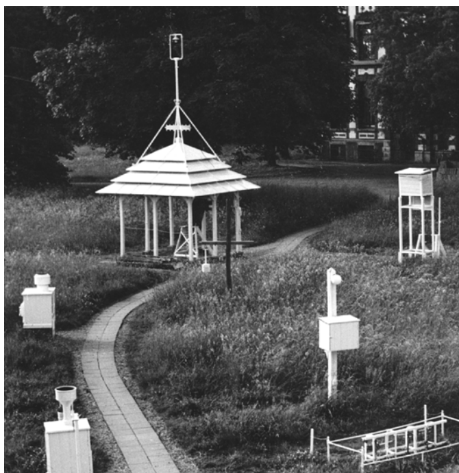
Figure 2: Screen change in De Bilt on 16 September 1950. On the left the old pagode screen and on the right the new Stevenson screen.
