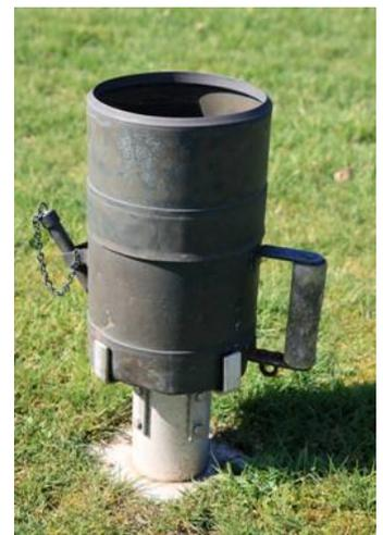
Figure 4: Example of a manual rain gauge (with the rim at 0.4 m).
