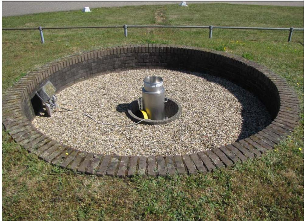
Figure 2: KNMI automatic rain gauge in English set-up.
