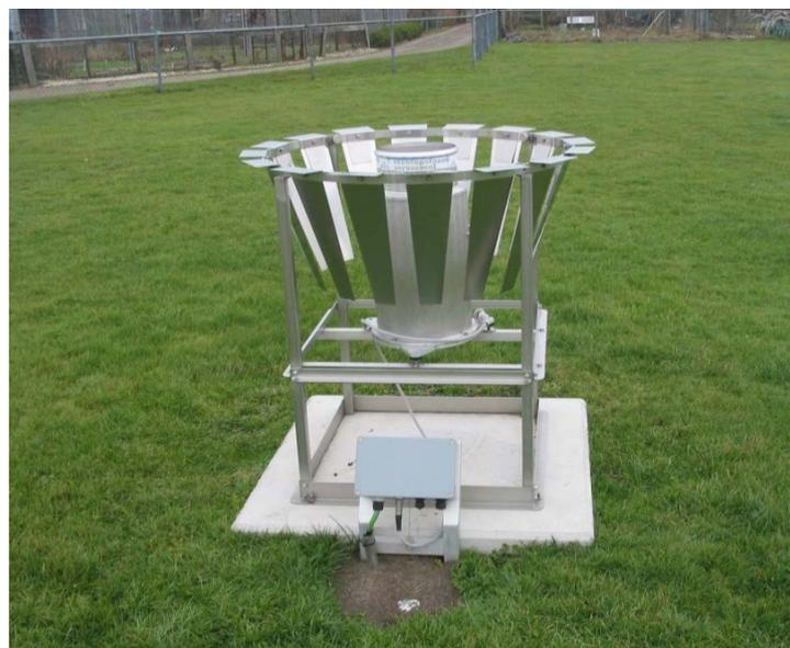
Figure 3: KNMI automatic rain gauge in an Ott screen.
