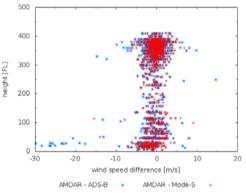
Figure 23: Wind speed difference of AMDAR and Mode-S EHS (red crosses) and ADS-B EHS (blue stars), respectively versus height.
