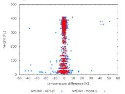
Figure 22: Temperature difference of AMDAR and Mode-S EHS (red crosses) and ADS-B EHS (blue stars), respectively versus height.
