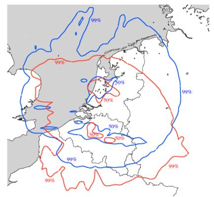
Figure 10 : Relative horizontal coverage of the total number of Mode-S EHS wind and temperature observations retrieved from ATC (blue) and ADS-B EHS (red) data during nine days (1-9 April 2012).
