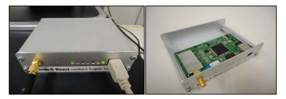
Figure 2 :The Mode-S Beast "Series 2" in operation (left) and the PCB inside the housing (right).
