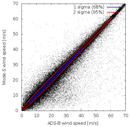
Figure 20: Comparison of Mode-S EHS and ADS-B EHS wind speed observations.
