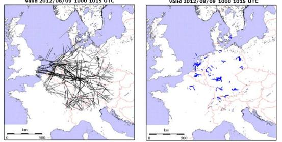
Figure 24: Example of 15 minutes of derived Wind and Temperature observations from Mode-S EHS data (quality controlled) of a day in August 2012 over Western Europe, source Maastricht Upper Area Control Centre (MUAC) of EUROCONTROL, processed by KNMI.
