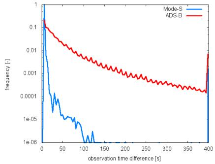
Figure 12: Frequency distribution of the time difference of subsequent wind observations from Mode-S EHS (blue) and ADS-B EHS (red).
