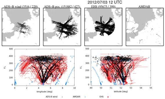
Figure 7: Example of the horizontal (upper panels) and vertical coverage (bottom panels) of meteorological upper air observations retrieved from Mode-S EHS via ATC The Netherlands (labelled EHS), Mode-S EHS from the local receiver (labelled ADS-B wind) and AMDAR.
