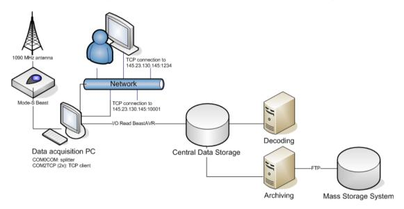
Figure 1 : Schematic overview of the Mode-S Beast data acquisition chain.
