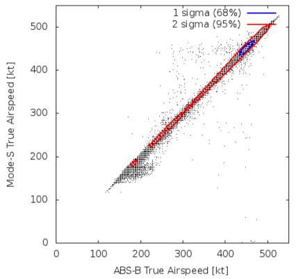
Figure 14 :Comparison of true airspeed observations from ADS-B EHS and Mode-S EHS.
