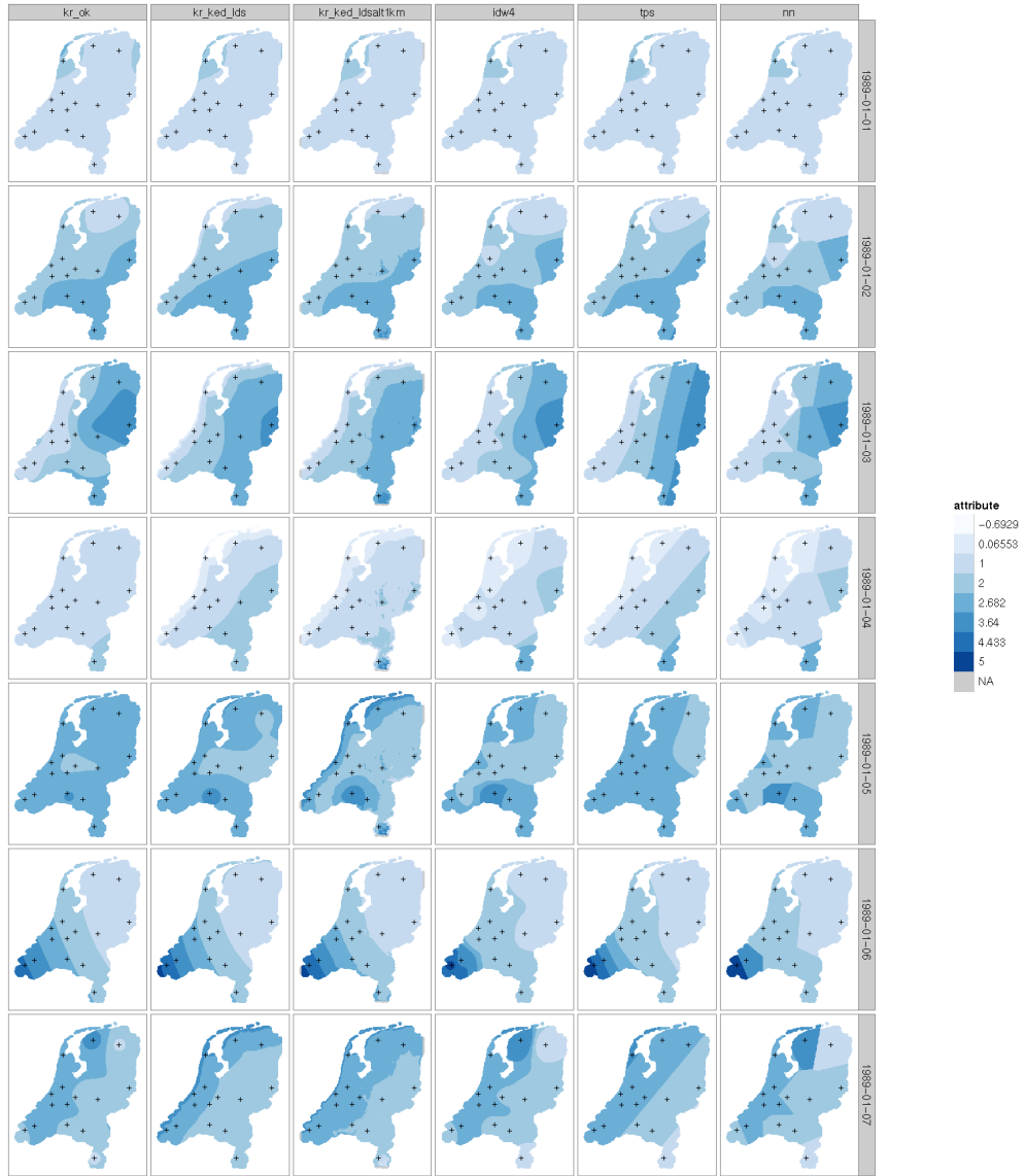
Figure B.3: Interpolated maps of daily Makkink evaporation ( 10^{-1} mm) for the first week of January 1989. Columns represent different interpolation methods, rows represent time.
