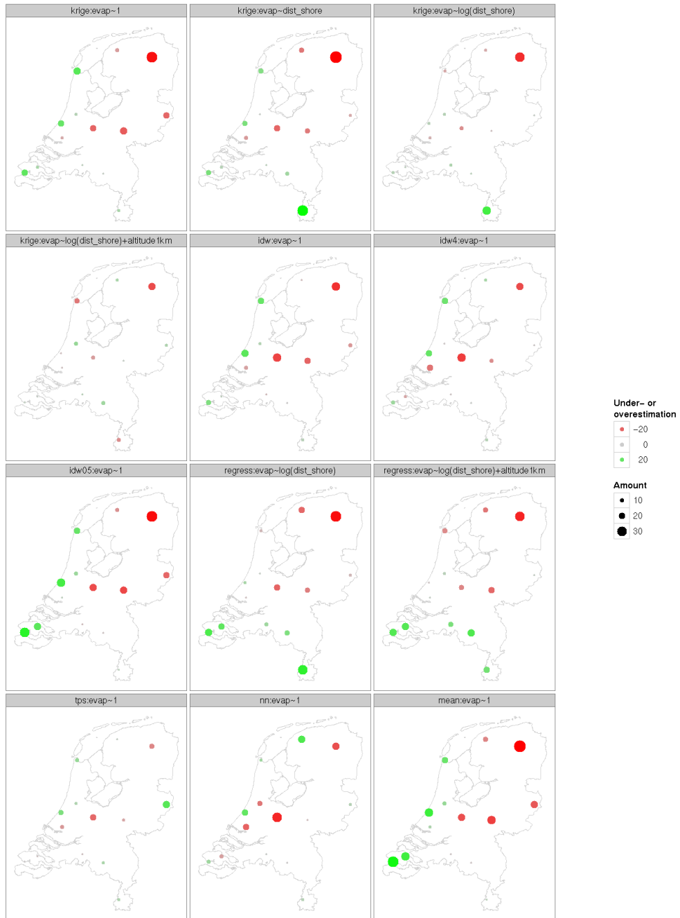
Figure 3.4: Map of the cross-validation residuals for all interpolation methods considered. Red is overestimation, green is underestimation.
