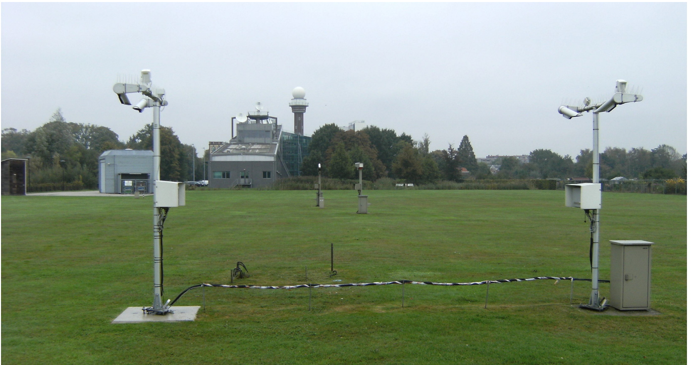
Figure 3: Field evaluation setup in De Bilt showing the emitter and short baseline receiver of the TMM in the background and the operational FD12P (right) and FD12P with the MOR filtering firmware (left) in the foreground.
