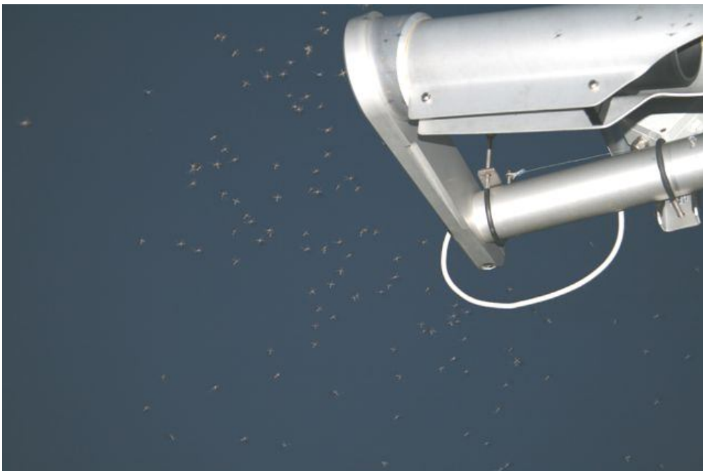
Figure 1: Example of the MOR reduction of the FD12P by insects observed in De Bilt on September 18, 2008 (a) and a picture showing insects around the FD12P on September 8, 2008 during a similar MOR reduction event (b).
