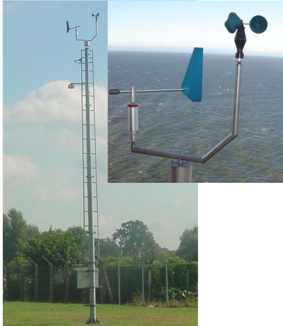
Figure 1: Picture of the KNMI cup anemometer and the wind vane as well as the standard measurement setup using a 10m mast at the test site in De Bilt.
