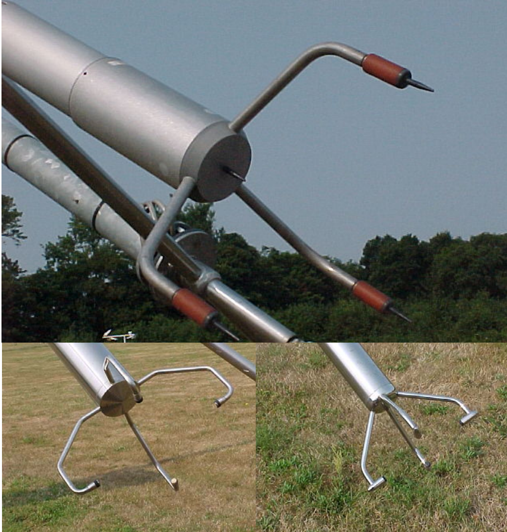
Figure 3: The Thies (lower left), Gill (lower right) and Vaisala (upper panel) sonic anemometers.
