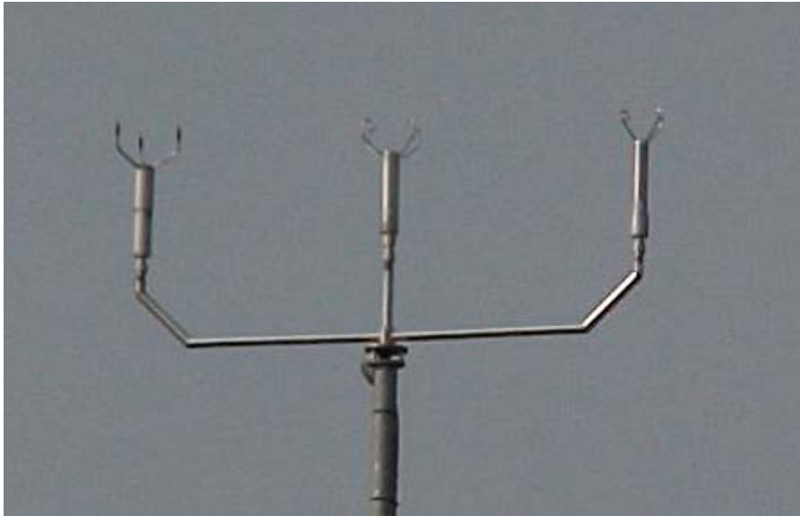
Figure 4: The cross arm on top of the 10m mast with the 3 sonic anemometers during the field test.
