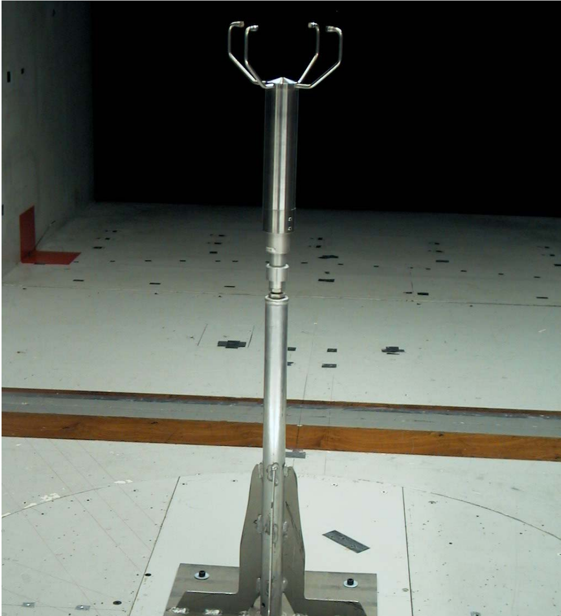
Figure 5: The Thies sonic anemometer situated on the monopod in the LST wind tunnel. Note the arc of the turntable in the floor.
