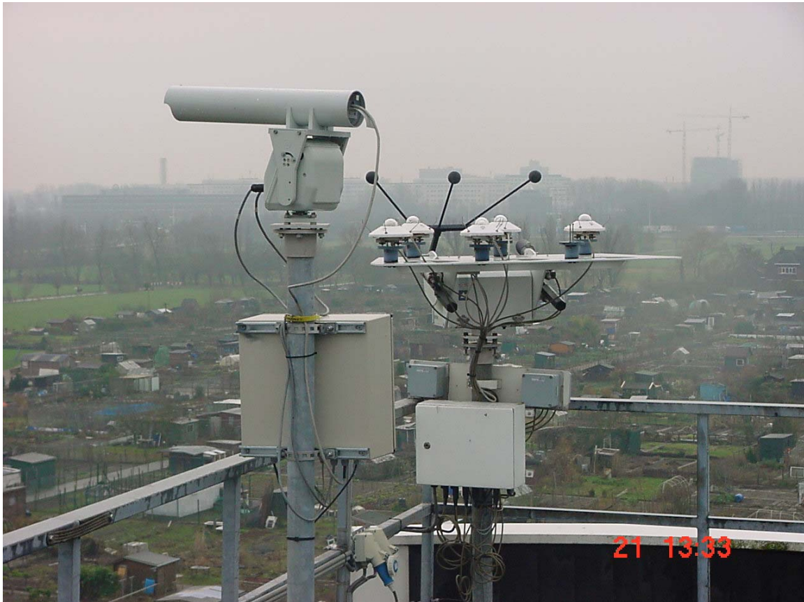
Figure 2: The Nubiscope system on the radiation platform during the test in De Bilt with a view to the South-East.
