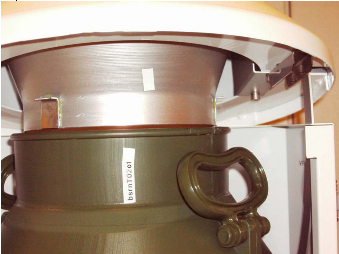
Figure 23: Photograph of the collector of the VRG101 sensor and the housing.
