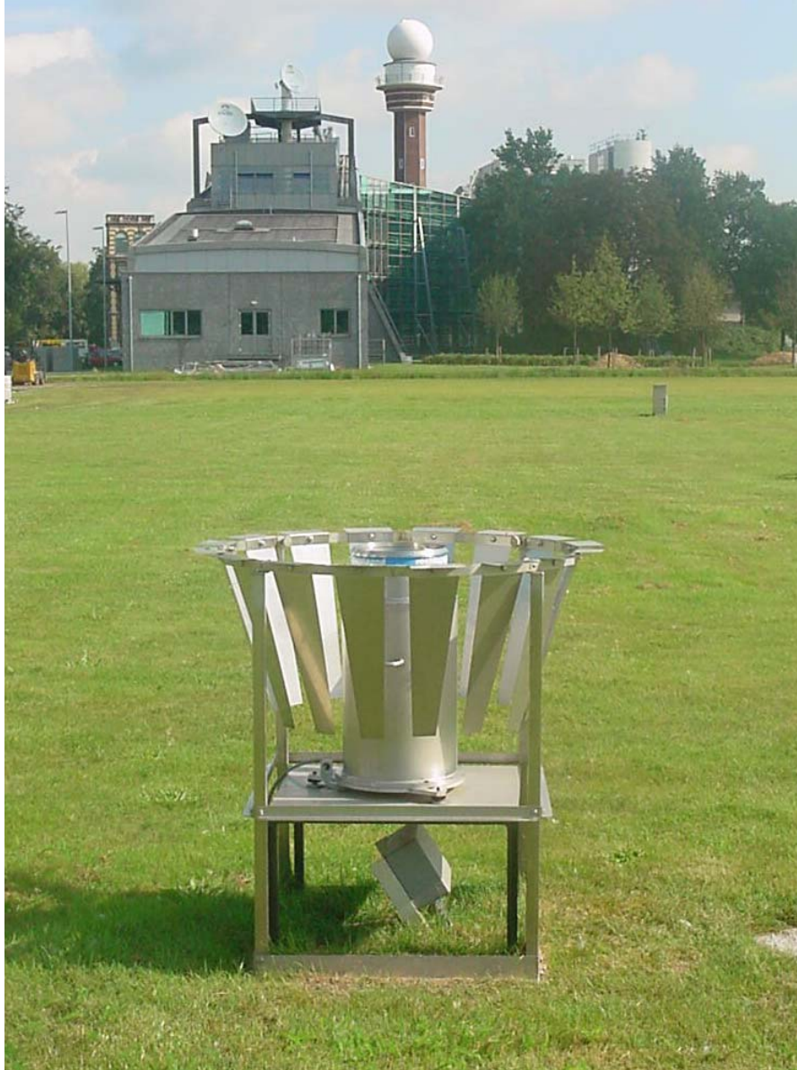
Figure 4: Picture of the precipitation amount measurement setup on the measurement field with a KNMI precipitation gauge within an Ott windscreen. In the background the main building of KNMI located to the North-Northeast of the measurement field.
