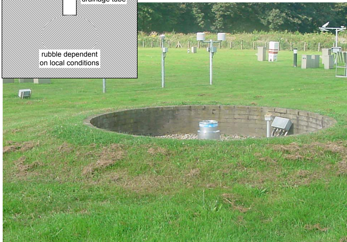
Figure 3: Schematic drawing of the so-called English setup used by KNMI for precipitation amount measurements. The photograph shows the English setup at De Bilt with in the background the trees Southwest of the measurement field.
