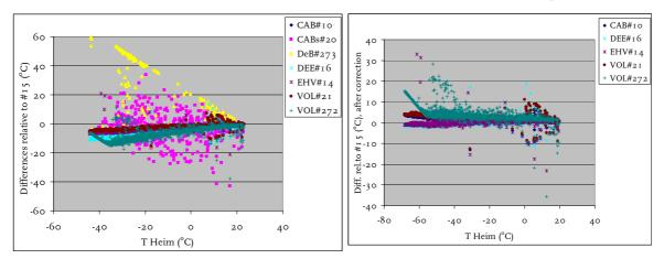
Fig. 7. Comparison of sky-looking Heimann infrared thermometers after the BBC1 experiment. In the right hand figure the data have been corrected, and data of Heimann #20 and #273 sets were omitted. Data represent 10 min averages.
