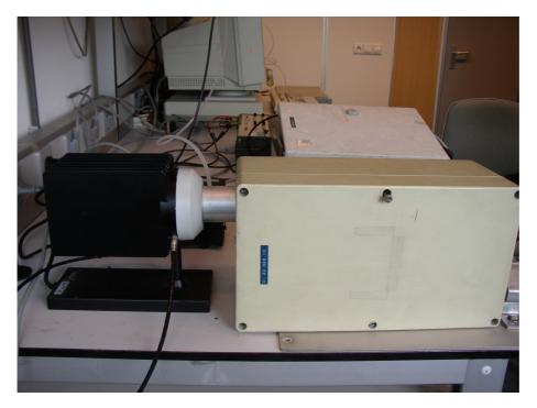
Fig. 1. Calibration set-up using the Galai black body (left). The Heimann is inside the thermostatted box on the right. In between the aluminium cylinder.
