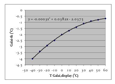
Fig. 2. Temperature difference between the Galai display the thermocouple, with regression curve.
