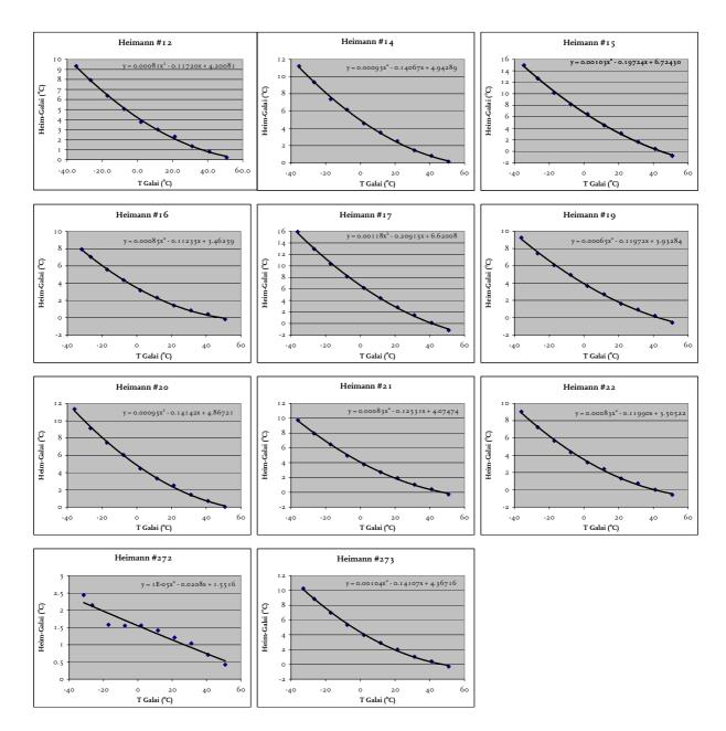
Fig. 6. Calibration results. Note that the abscissa is here the corrected Galai temperature, which leads to regression coefficients that are different from the calibration coefficients of Table 1.
