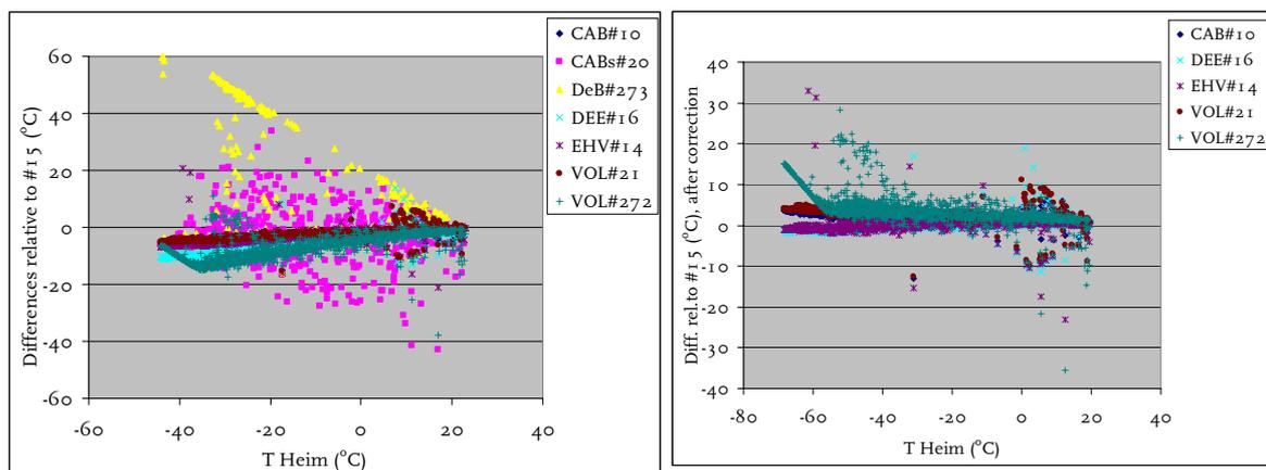
Fig. 7. Comparison of sky-looking Heimann infrared thermometers after the BBC1 experiment. In the right hand figure the data have been corrected, and data of Heimann #20 and #273 sets were omitted. Data represent 10 min averages.
