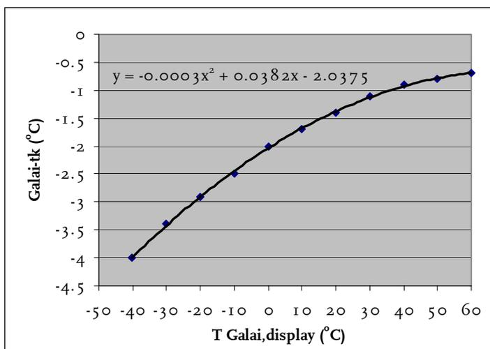
Fig. 2. Temperature difference between the Galai display the thermocouple, with regression curve.
