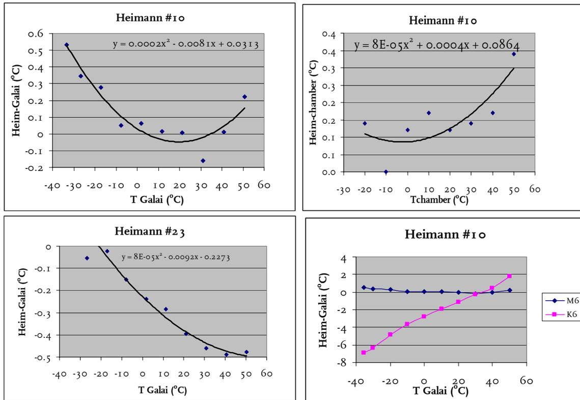
Fig. 3. Above and below left: difference between the reading of the Heimann and the Galai black body or climate chamber, after repair. Below right: effect of lens type. The Galai temperature has been corrected.
