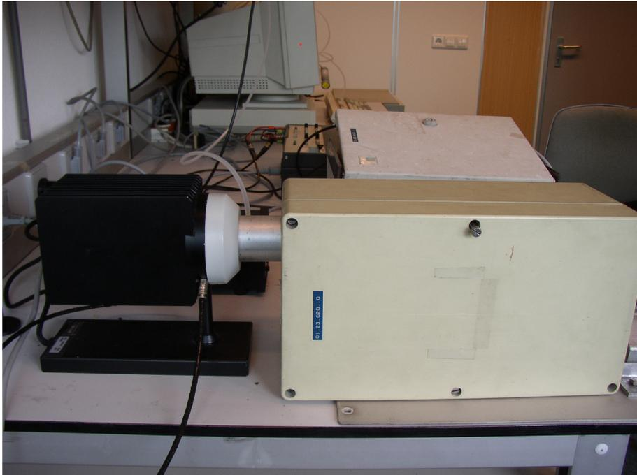
Fig. 1. Calibration set-up using the Galai black body (left). The Heimann is inside the thermostatted box on the right. In between the aluminium cylinder.
