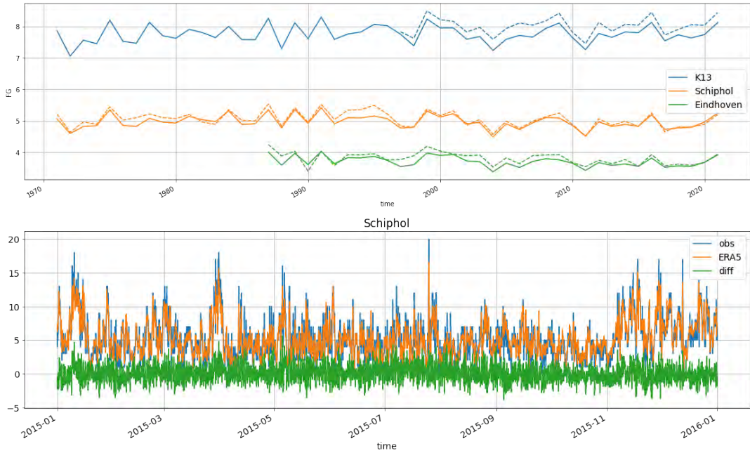
Figure 3.23: Comparison between observed (KNMI uurgegevens, 2023) and reanalysed (ERA5) wind speeds. Upper panel: Annual-means at two land and one sea station. Continuous line ERA5, dashed line observations. Lower panel: One year (2015) of hourly wind speeds and their difference at station Schiphol.
