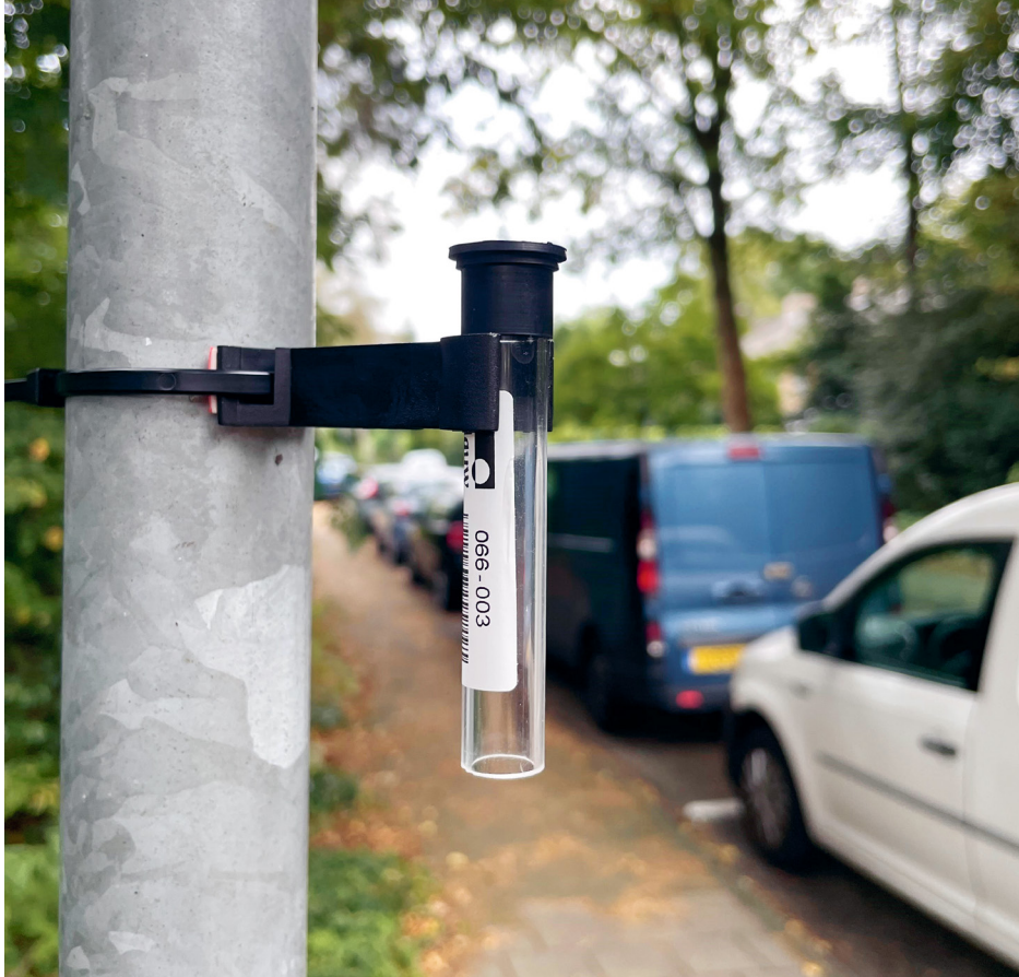
Figure 2. Palmes tube mounted on a lamp post (right). Photos: GLOBE
