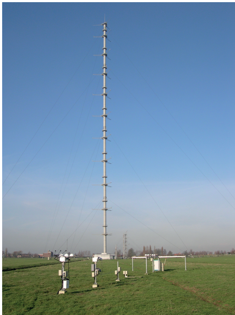
Cabauw Experimental Site for Atmospheric Research (CESAR). In front KNMI's Baseline Surface Radiation Network site. At the back, the Cabauw observation tower. Photo courtesy: Wouter Knap
