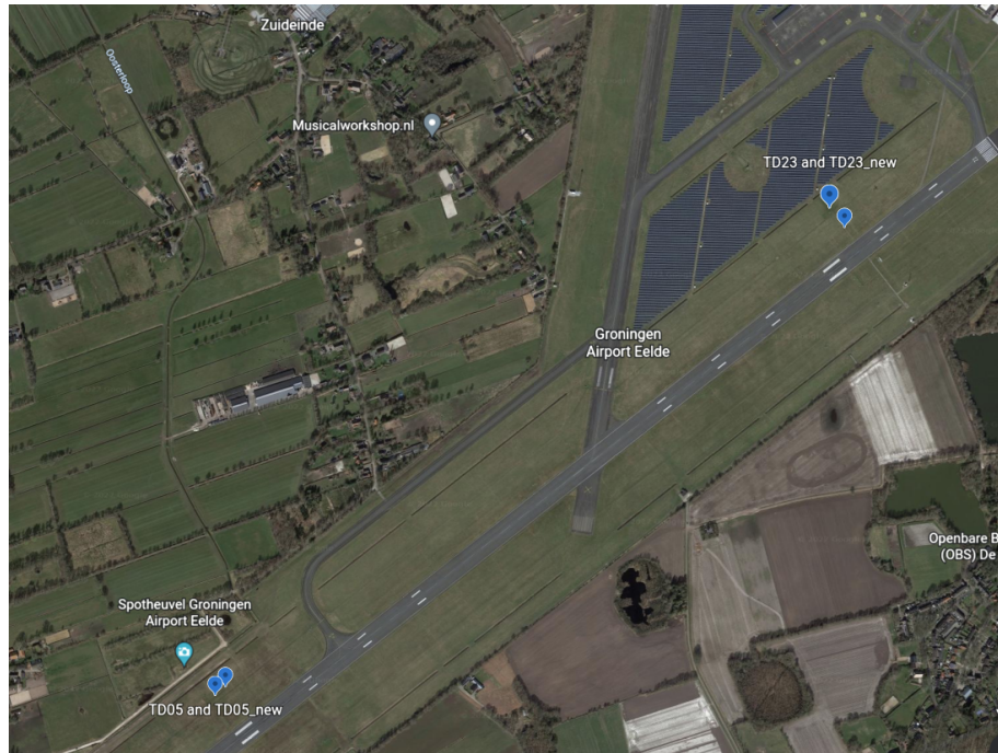
Figure 1.1: Map of Groningen Airport Eelde after installation of the solar farm. TD23 is the operational location, TD23_new is an alternative for TD23 that may replace TD23 in the future. TD05 is the backup location and TD05_new is situated just East of TD05 because of the shadow effect of the wind mast. The distance between TD23 and TD05 is about 1.6 km
