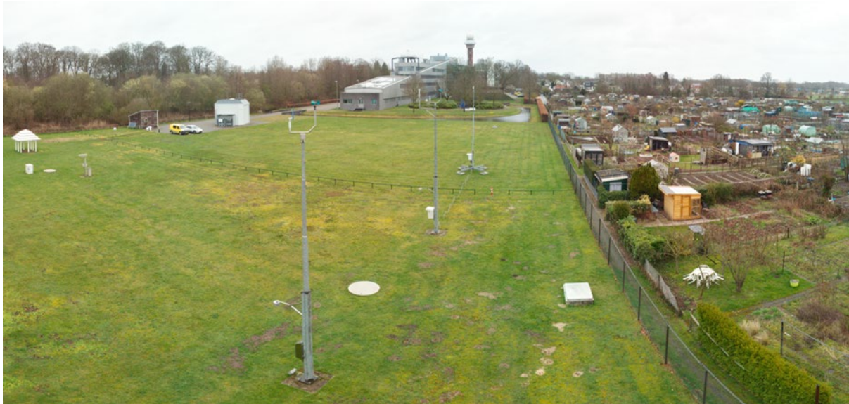
Figure 2: Part of a panorama photo of the test site taken at 10 m height, looking north. The closest mast (the most southerly) is not used in this study, the mast in the middle is the fixed mast with a cup anemometer and an old vane. The furthest mast is the mobile mast containing both a new and old vane. All measurements were made at a height of 10 m.
