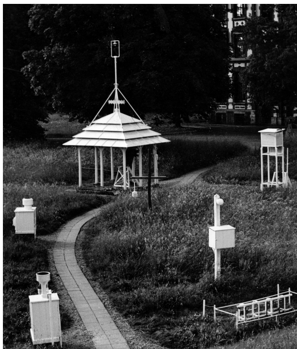
Figure 2.6: Screen change in De Bilt on 16 September 1950. On the left the old pagoda screen and on the right the new Stevenson screen. Note that this Stevenson screen is still at 2.20 m above ground level and not at the current 1.50 m (see Section 2.4).
