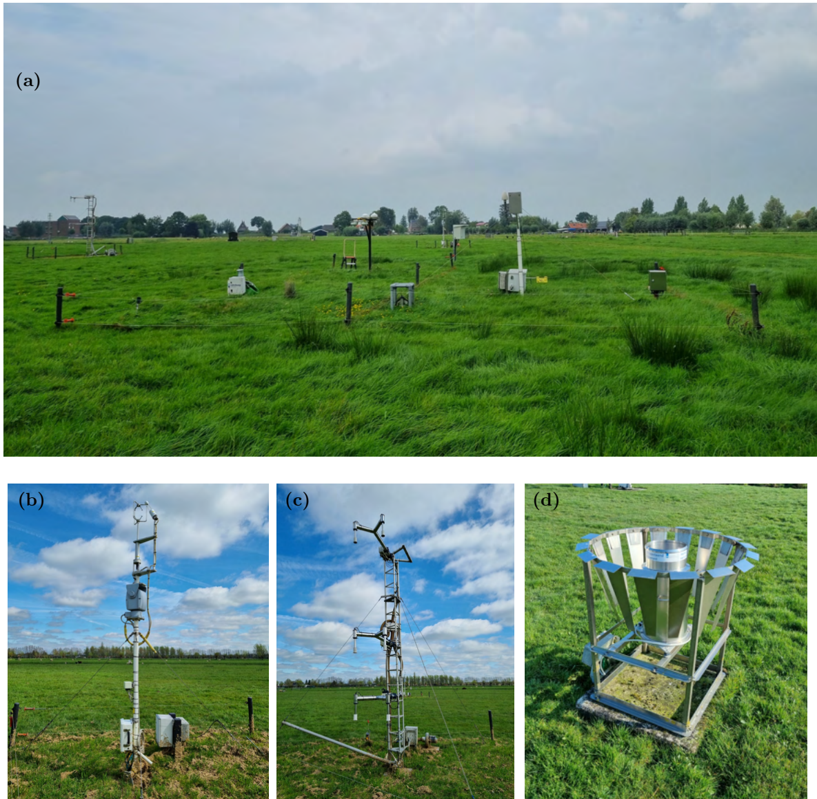
Figure 2: (a) Energy balance field with a variety of related instruments described in Reference [6]. (b) Turbulence measured at 3 m height using a 3D sonic anemometer and open path sensor installed together on a rotator which aligns with the wind direction. (c) Psychrometer measuring both the air and dew-point temperature at 1, 2 and 4 m. (d) KNMI precipitation gauge located at the automatic weather station near the main mast.
