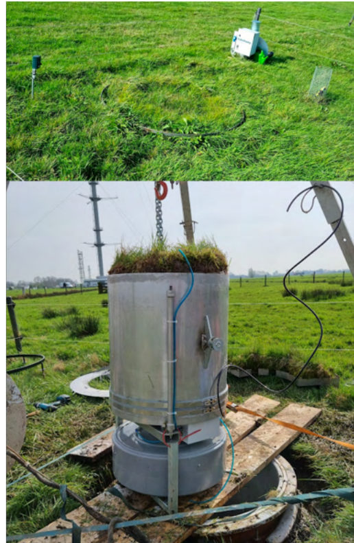
Figure 1: Upper: Top-view of undisturbed lysimeter plot with external tensiometer located on the far right. Lower: Unearthed lysimeter showcasing the soil column and lower reservoir.
