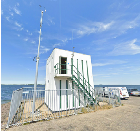
Figure F.28: Stavenisse/Tholen (324): wind measurements are too disturbed by 5 m tall building next to the wind mast.
