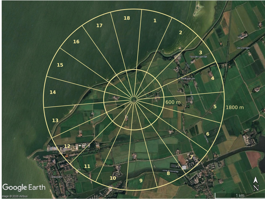
Figure F.15: Directional sectors around the wind mast at Stavoren (267).
