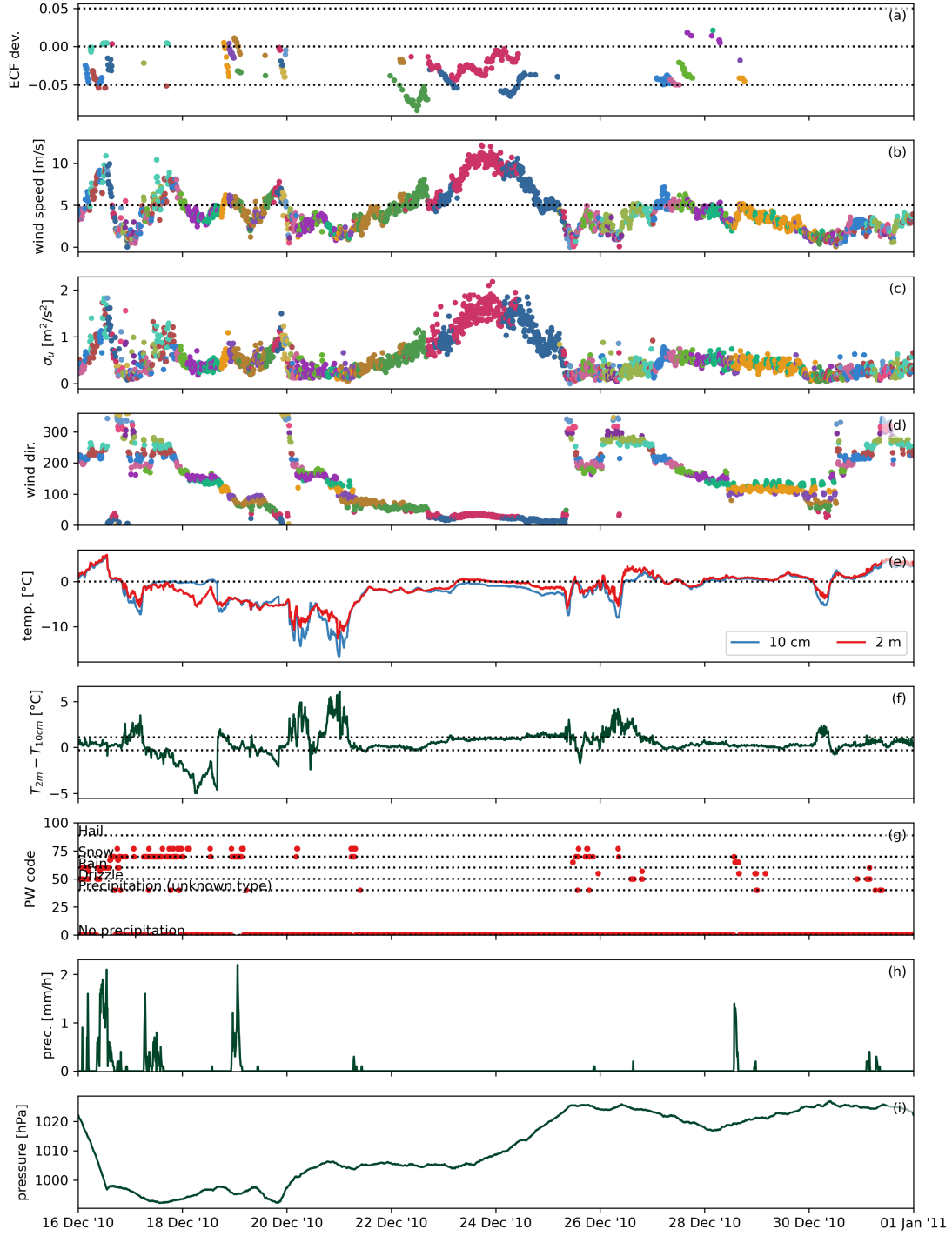
Figure 9: Deviations of ECF values from long-term average and a number of meteorological parameters for a case with snow at Schiphol: (a) ECF deviations with optimal filtering, (b) wind speed, (c) wind-speed standard deviation, (d) wind direction, (e) temperatures at 10 cm (blue) and 2 m (red), (f) temperature difference between 2 m and 10 cm, (g) present-weather code indicating precipitation type, (h) precipitation intensity and (i) pressure. The colours in a–d indicate the wind-direction sector.
