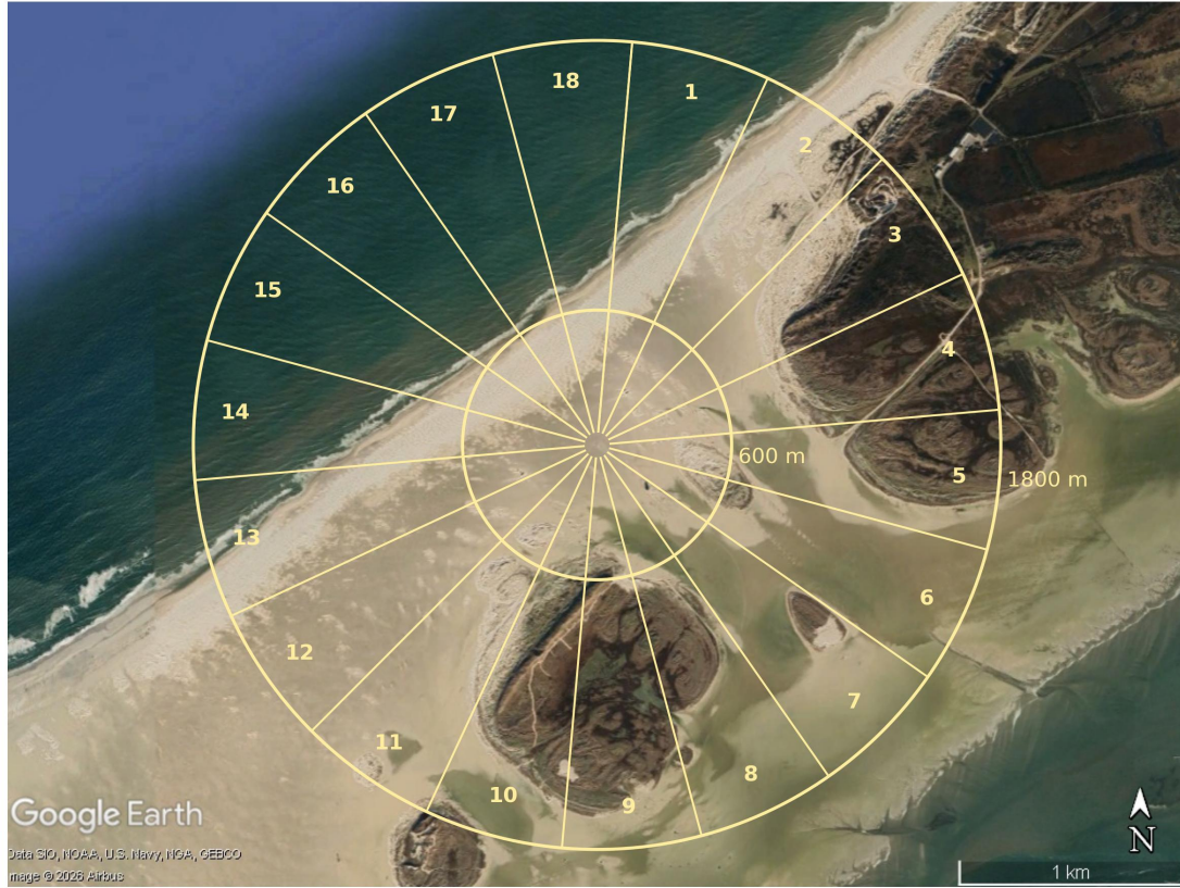
Figure F.8: Directional sectors around the wind mast at Vlieland Vliehors (242).
