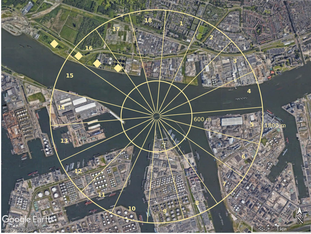
Figure F.30: Directional sectors around the wind mast at Rotterdam Geulhaven (343). Squares mark the positions of wind turbines.
