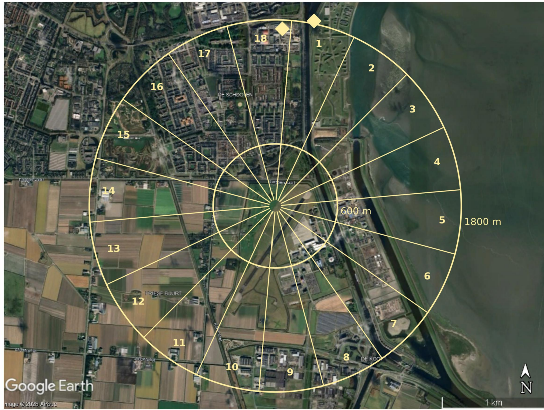
Figure F.7: Directional sectors around the wind mast at De Kooy (235). Squares mark the positions of wind turbines.
